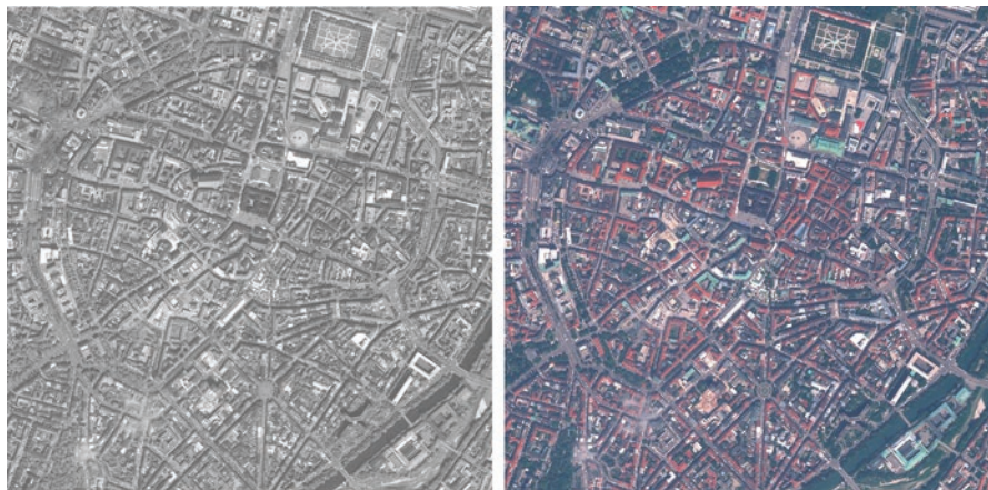
Fig. 16 Section 1.75 \times 1.75 \text{ km}^2 , Munich city center, left, panchromatic “left” image; right, multispectral (red, green, blue) “left” image
