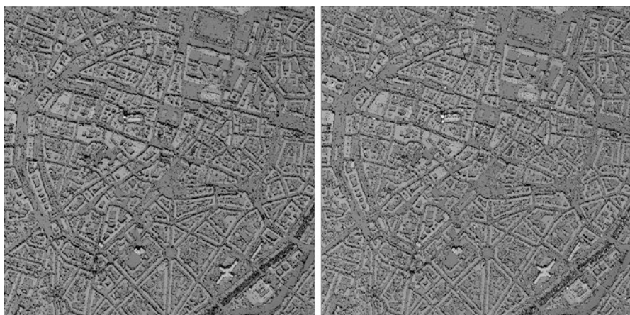
Fig. 18 Section 1.75 \times 1.75 \text{ km}^2 , Munich city center, left, height map fitting on left original image; right, final DSM, UTM zone 32 north, WGS84 ellipsoid
